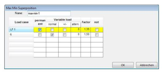
You can calculate only one single max./min. superposition at a time. When you enter an additional max./min. superposition it will overwrite the previous one.
