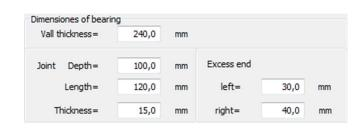
For Neoprene supports, the permissible tension [N/mm²] is prompted in addition ("permissible=").
