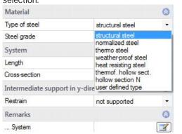
Steel grade the available options for the steel grade depend on the selected steel type.
