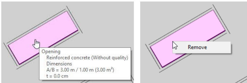
Fig. : With a "right click" on an opening, openings (both in walls and ceiling tiles) can be removed.
