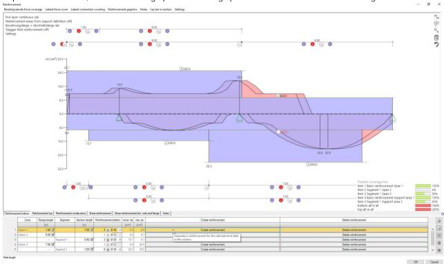
The reinforcement layout is generated on the basis of the tensile force or shear force coverage diagram. For T-beams, a required shear and, if necessary, shoulder shear coverage is also taken into account. Moreover, you can reinforce cut-outs existing in the structural system. Optionally, you can lay the required reinforcement in the section.
