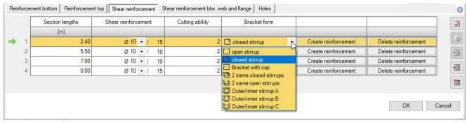
Double-shear and quadruple-shear stirrups are available as reinforcement
