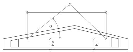
The default setting for HIe and Hri is the corresponding girder top edge. If a suspension lug projects considerably over the girder top edge, you should consider its elasticity via a reduction in height of the suspension points.
