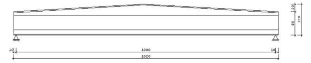
*III.:* Constant web height: the height of the webs is constant, the thickness of the top flange varies over its length.
