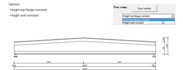
III.: Constant top flange: the thickness of the top flange is constant over its total length.
