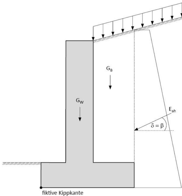
$$M_{G,k,dst} \cdot \gamma_{G,dst} + M_{Q,rep,dst} \cdot \gamma_{Q,dst} \leq M_{G,k,stab} \cdot \gamma_{G,stab}$$
